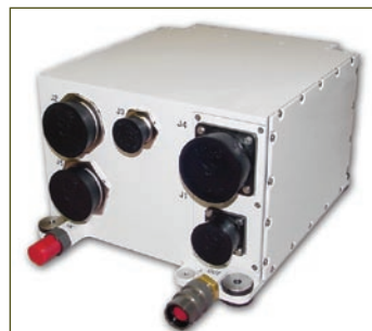
Figure 1 | Curtiss-Wright Controls Electronic Systems' family of rugged, high-efficiency SMCs, packaged as LRUs for vetronics applications.
